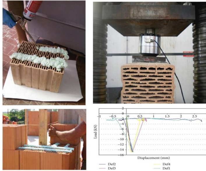
Figure 1. Effect of using polyurethane foams in masonry on mechanical properties (Foti et al., 2018)
